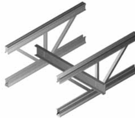
Standard strongback installed on vertical webs.
