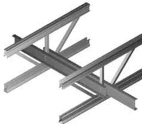
Strongback splice - overlap one truss as shown.
