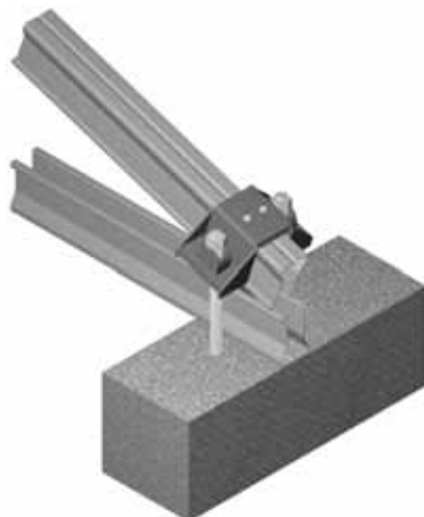
TrusSteel truss anchored to concrete bearing using ITWBCG Hardware GTH-series connector and epoxy-installed threaded rod.
