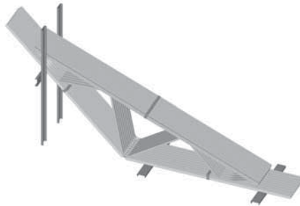
Vertical storage using a rack or stand. Always stake trusses to prevent toppling.
