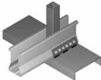
Welded connection to CFS using WTC Clip
